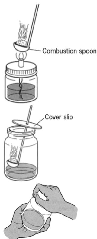
Fig. 6.6: Burning non-metals in air
