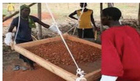
Fig. 5.3: Using a sieve to separate stones
