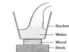
Testing the compression strength of your bricks
